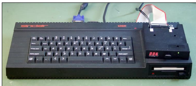
And this is what it looks like - the Gotek at the Spectrum +3
